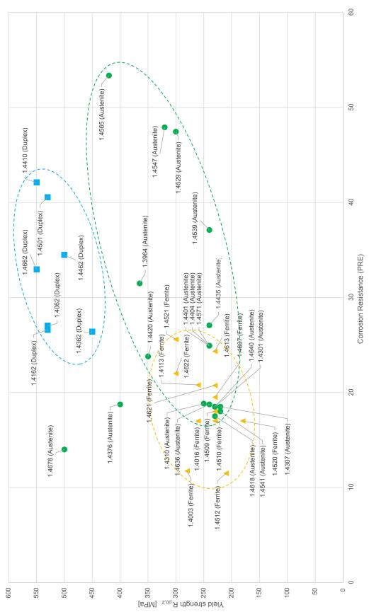
PRE: Pitting Resistance Equivalent Number of the respective grade, calculated from the arithmetic mean of the limits for the alloying elements given in DIN EN 10088-1:2014-12.
