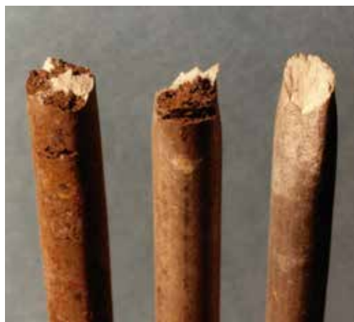
Figure 7: Serious accident in the indoor swimming pool in Uster (Switzerland) in 1985, in which numerous people died due to the collapse of the suspended ceiling. The cause was stress corrosion cracking on the Cr-Ni steel (CRC II) suspension brackets. The surfaces of the broken brackets show varying degrees of advanced corrosion. The bracket on the right shows severe necking with a typical sliding fracture surface and has probably borne the longest. A slight necking is still visible on the middle bracket.
