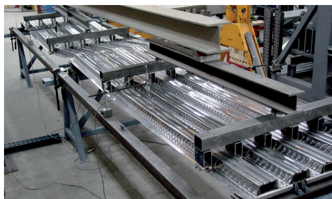
Figure 9 Continuous decking tests at the construction stage
