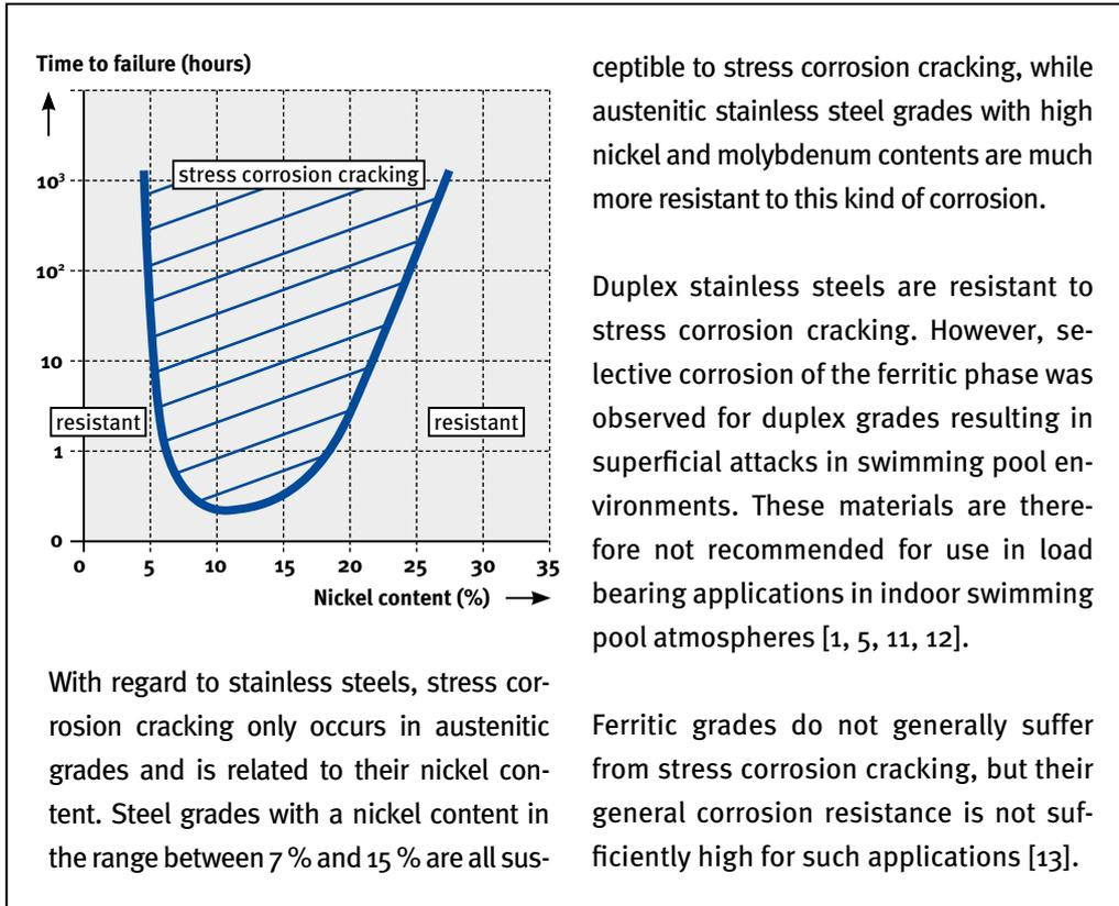
Structural engineers and pool operators are advised to take some practical measures to prevent stress corrosion cracking which have proven useful over many years.
