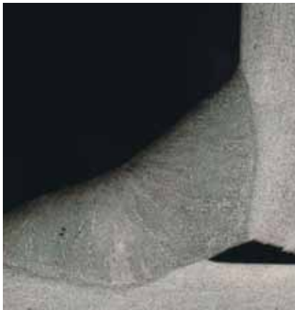
The section shows a rather low and asymmetrical penetration form.
