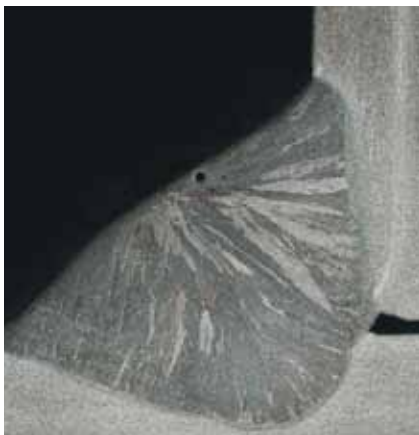
The section shows a slightly convex reinforcement. This geometrical form might reduce fatigue performance. Close to the weld surface, there is slight porosity. This is typical of this procedure.
