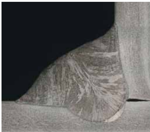
The section shows a rather convex reinforcement.
