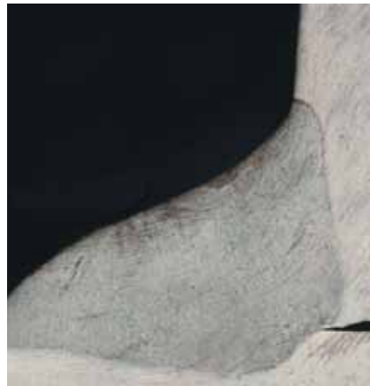
The section shows a relatively convex, asymmetrical reinforcement.
