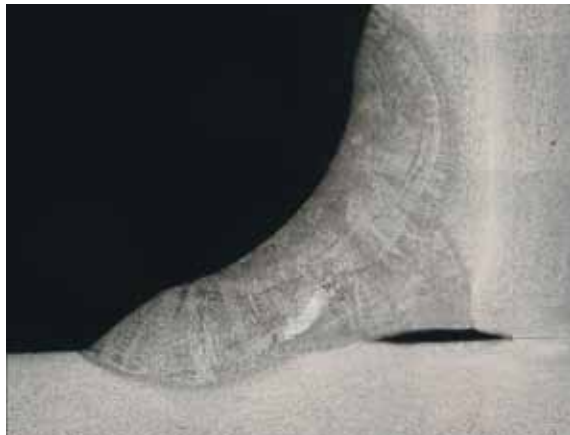
The section shows a concave weld.
