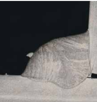
The section shows a convex reinforcement. The use of higher voltage would have reduced the convex profile. On the surface, a small amount of spatter appears. This is typical of this procedure.
