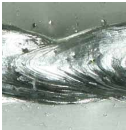
The section shows a slightly convex reinforcement. This geometrical form might reduce fatigue performance. Close to the weld surface, there is slight porosity. This is typical of this procedure.
