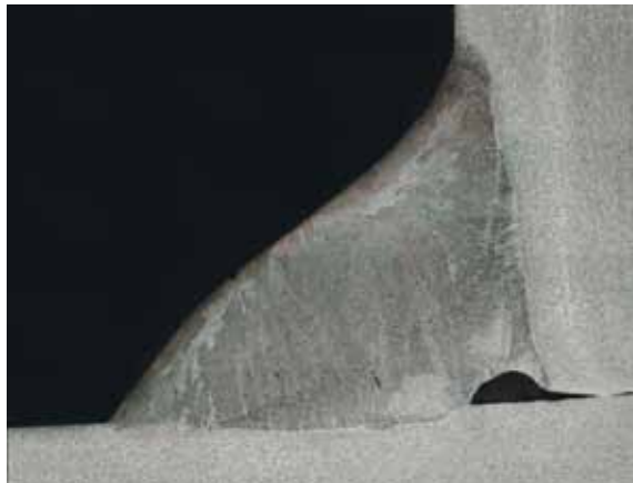
The section shows a rather convex/flat reinforcement.
