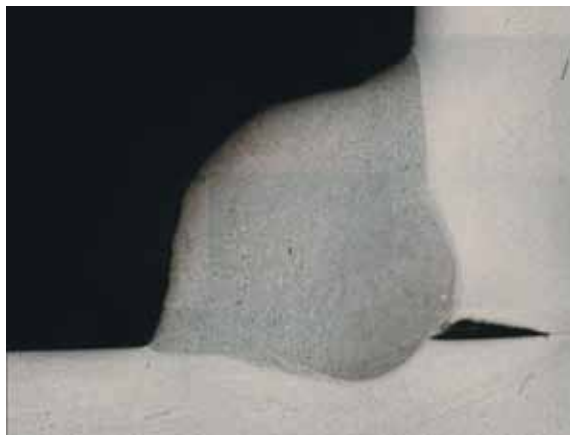
The section shows a convex weld. This is typical of this procedure.
