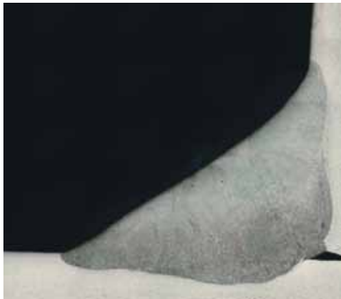
The section shows good concave/flat reinforcement.
