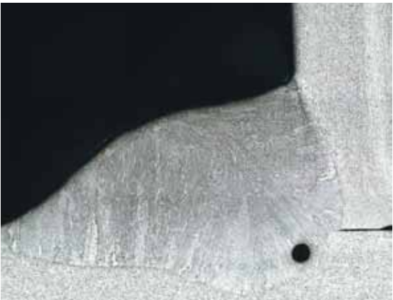
The section shows a rather asymmetrical and convex reinforcement. On the root side a typical porosity appears.
