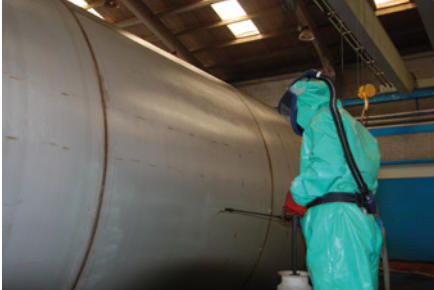
Spray pickling is an option for components that are too large for immersion treatment. Photo: Vecom, Maassluis (NL)
