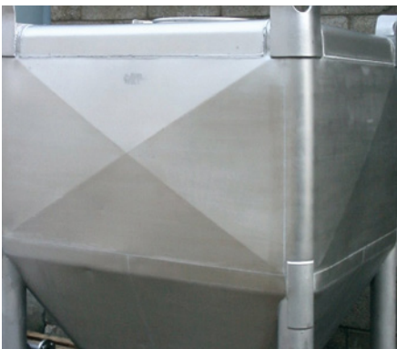
Passivation also has a cleaning effect and removes iron contamination which may have occurred in a mixed-material workshop. Photo: Edward Uittenbroek, Gouda (NL)
