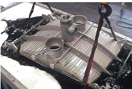
Chemical surface treatment by immersion creates optimal conditions for consistent results. Photos: Edward Uittenbroek, Gouda (NL)
