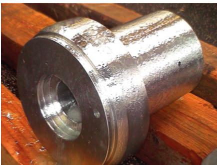
For occasional use, smaller parts or local treatment, pickling paste is a practical solution. Photo: Edward Uittenbroek, Gouda (NL)
