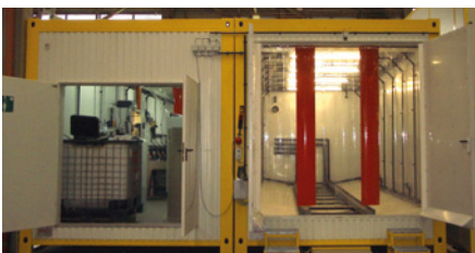
Transportable modular units create a safe, enclosed environment for the chemical surface treatment of metals. Photo: Poligrat, Munich (D)
