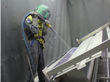
Blasting is often preferred to produce uniform finishes on larger assemblies Photo: Centro Inox, Milan (I)
