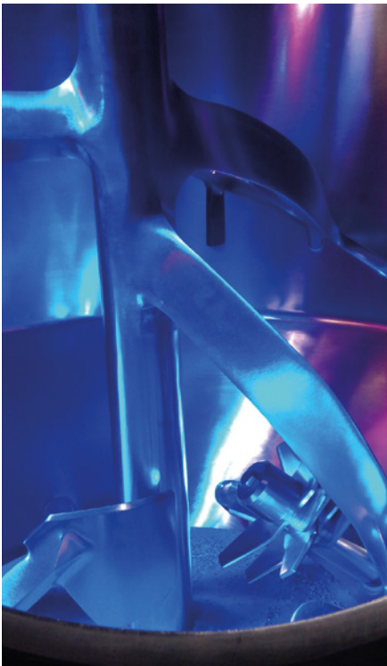
Only clean metallic surfaces create the necessary conditions for the passive layer to form properly on stainless steel.
