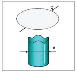
LDR values are improved compared with the classic 1.4372 (201) grade. The combination of minimum 1 % Cu additions and optimum nitrogen content obviously significantly improves the formability properties of grade 1.4618 compared to other 200 series grades.
