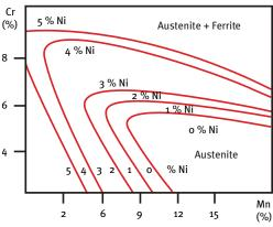
Figure 2. Alloying elements and austenite loop stability at 1075 °C (Franks)
