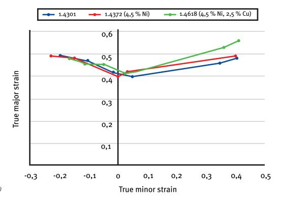
Figure 12. Forming limit diagram (thickness 1 mm)
