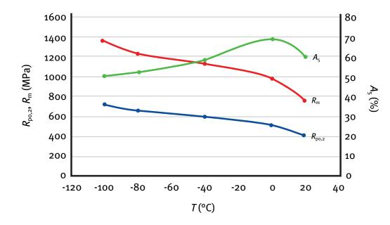
Figure 5. Mechanical properties at sub-zero temperatures for 1.4372 (N = 20, thickness 2 mm, Ni 3.6-4.5 %, C 0.03-0.06 %)
