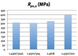
sensitive to martensitic phase transformation than CrNi austenitic grade 1.4307.
