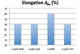
Figure 4. Comparison of the mechanical properties of several austenitic stainless steels at room temperature (2B, 3 mm)
