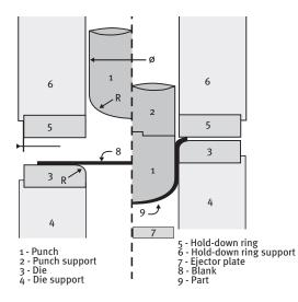
Figure 8. Stretchforming (left) and drawing process (right)
