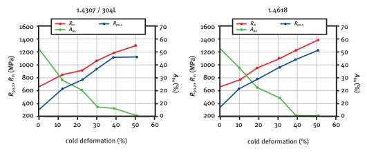
Figure 3. Mechanical properties versus cold deformation for 1.4307/304L (left) and 1.4618 (right)
