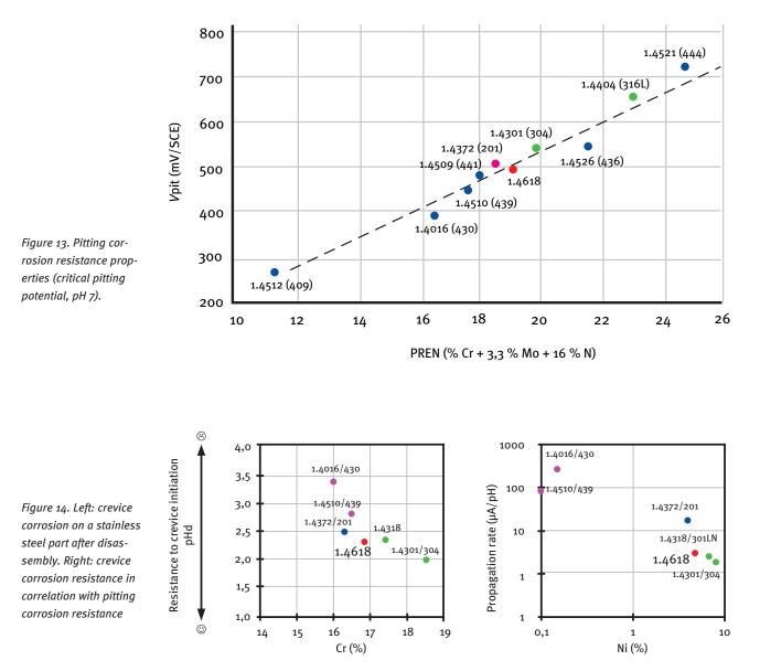
The crevice corrosion resistance (crevice initiation) of grade 1.4618 is significantly better than that of other 200 series grades. It is equivalent to that of 1.4310 (301) and very close to grade 1.4307 (304L).
