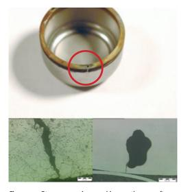
Figure 15. Stress corrosion cracking on the cup after testing
