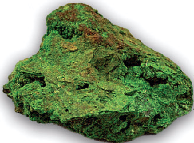
Nickel ore: Garnierite (New Caledonia) – Courtesy of Ecole des Mines de Paris
