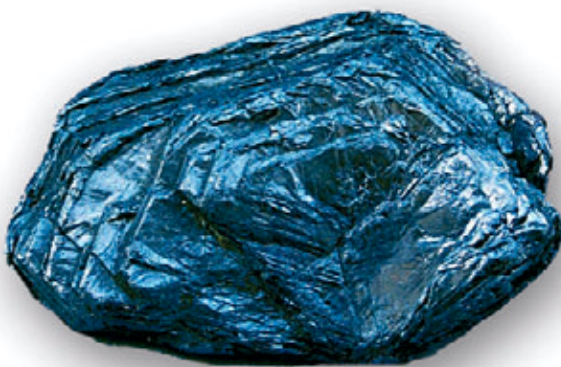
Molybdenum ore: Molybdenite – Noerkheia (Norway) – Courtesy of Ecole des Mines de Paris
