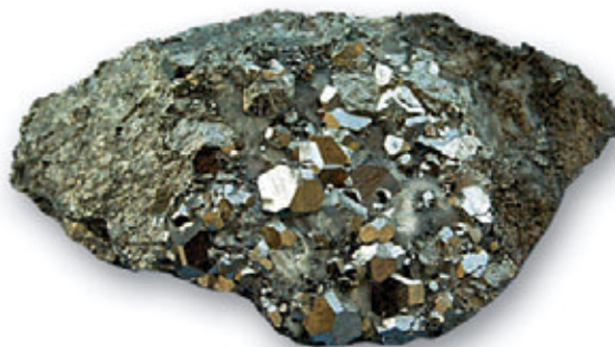
Cobalt ore: Skutterudite – Irhtem (Morocco) – Courtesy of Ecole des Mines de Paris
