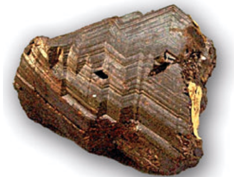
Titanium ore: Rutile - Parsksburg (USA) – Courtesy of Ecole des Mines de Paris
