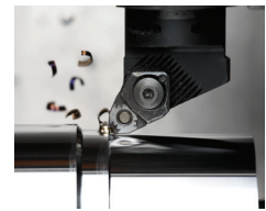
Photo 5: Coated carbide insert used in rough turning
