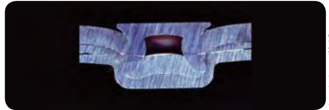
Auto-riveting on 430, 1.5 mm.
