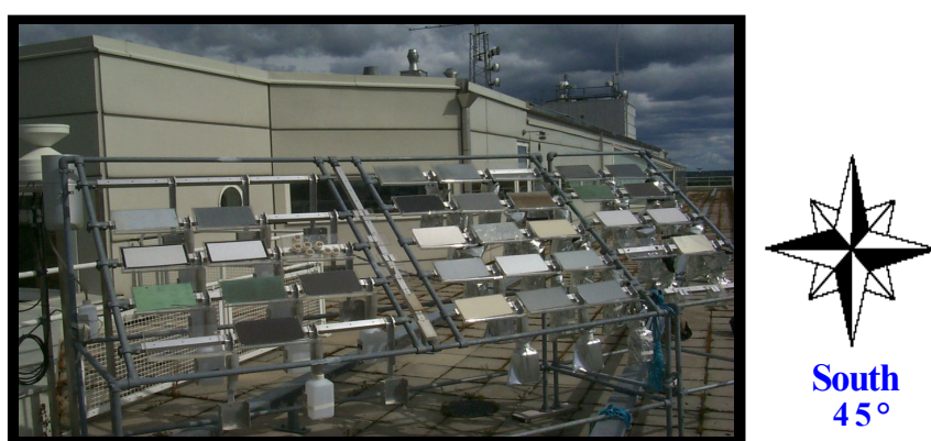
Fig. 7 Field exposure test site for metal release studies.
