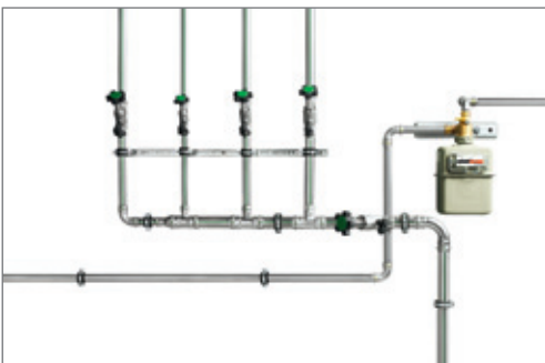
Stainless steel press fitting systems are equally suited to gases. Photo: Viega, Attendorf (D)
