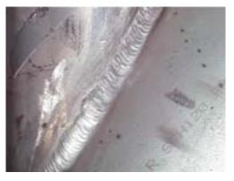
Detail of the welded area after chemical surface treatment: the purpose of this treatment is not to remove the weld seam itself, but the welding tint that accompanies it.
