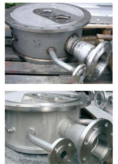
Heat tint left in welded areas of a complex fabrication can be effectively removed by pickling by immersion pickling. The corrosion resistance of the whole fabrication has been restored by pickling.
