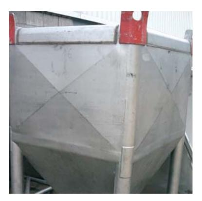
A fabricated hopper before surface cleaning & pickling, shows shopsoil, part number marks, painted areas and weld heat tint. If the surfaces are not properly treated before the hopper enters service, inadequate corrosion resistance could result in premature system failure. Passivation is covered by European Standard:
