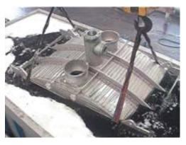
Tank immersion pickling: If the dimensions of the fabricated part match the tank dimensions, the complete part can be immersed in a tank for pickling. Immersion temperature and duration affect the result of the pickling process.
