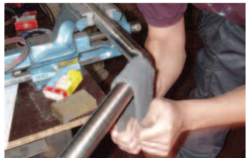
Hand finish blending the complete rail into one finish forming a smooth connection between the two tubes.
