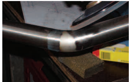
The complete perimeter of the joint can be pretreated with just flap discs abrasives.
