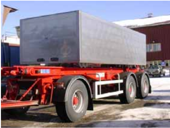
Figure 53. Stainless steel sandwich panels used as side and floor elements of a gravel trailer platform (Kenno Tech 2008).
