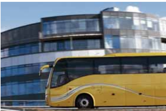
Figure 19. Coach with a stainless steel body frame and skin (Volvo Bus 2007).
