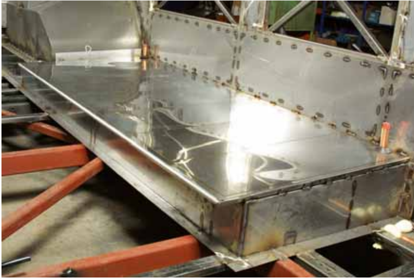
Figure 52. An experimental, sandwich-panel bus floor element, in grade 1.4003, assembled using laser welding (Alenius et al. 2002).
