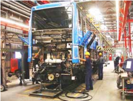
Figure 21. Assembly of buses with a stainless steel chassis and (ferritic) stainless steel skin (Centro Inox 2007a / De Simon 2007).
