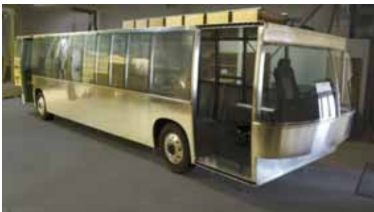
Figure 25. Rear view of an ultra-light, stainless steel, hybrid electric transit bus being developed under a DOE/industry partnership (Fisher 2008).
