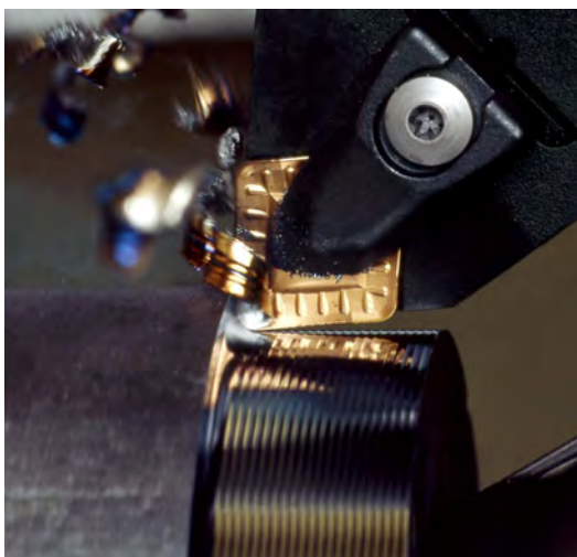
Turning stainless steel using carbide with a built-in chip breaker. (Source: Seco Tools)
