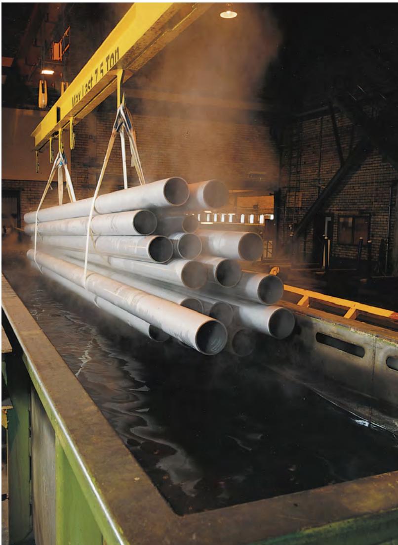
Degreasing of austenitic stainless steel. (Source: Sandvik)
