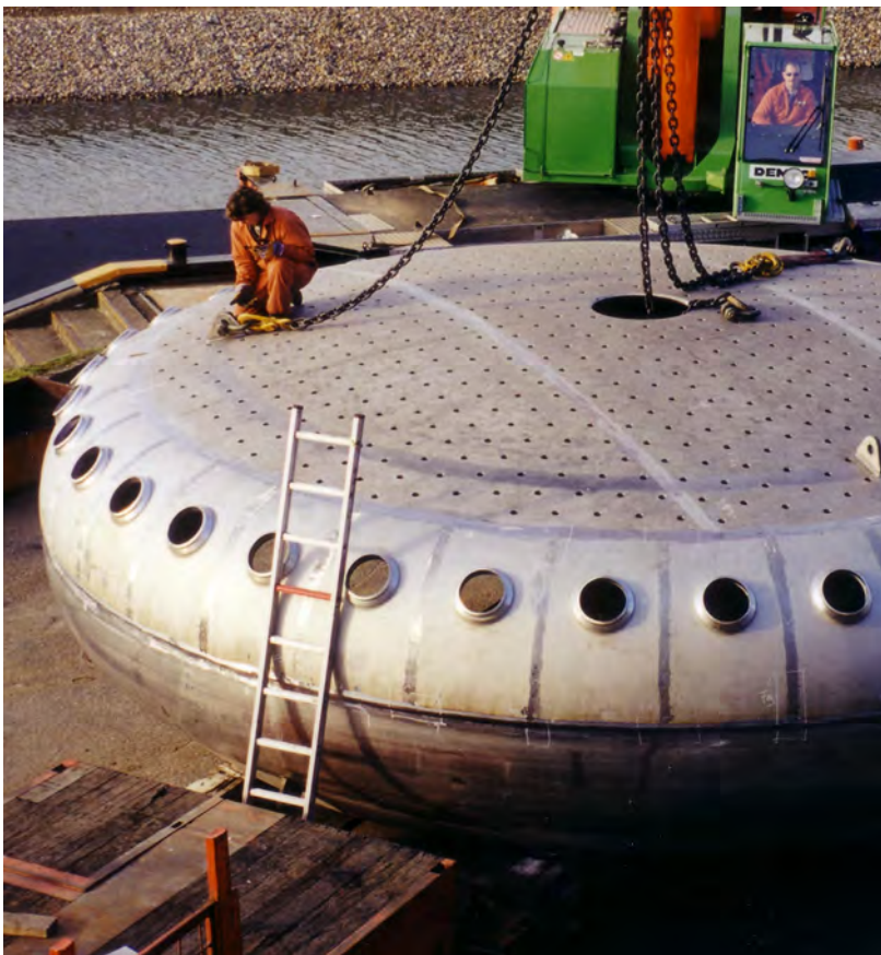
Large reactor head in austenitic stainless that has been weld fabricated from cold formed sections. (Source: Antonius Vesselheads BV)
