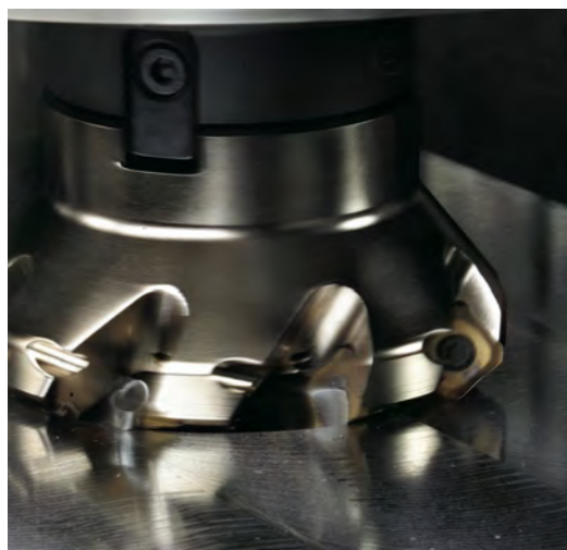
Face milling austenitic stainless steel with a carbide insert cutter. (Source: Seco Tools)
