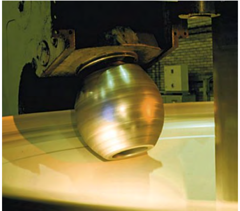
Spin forming of an austenitic stainless steel vessel head takes advantage of the steel's high ductility and low work hardening characteristics. (Source: Antonius Vesselheads BV)
