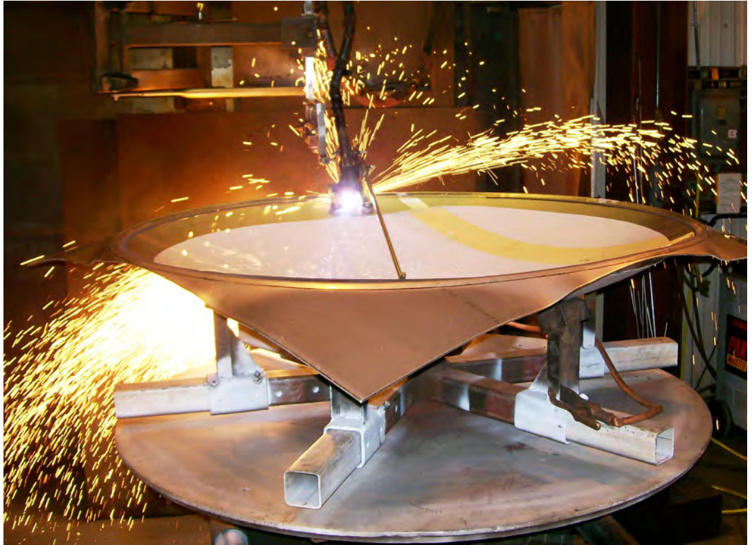
Plasma trimming of a GTA welded and hydro-formed austenitic stainless steel vessel head for sanitary applications. (Source: DCI, Inc, St. Cloud, MN USA)
