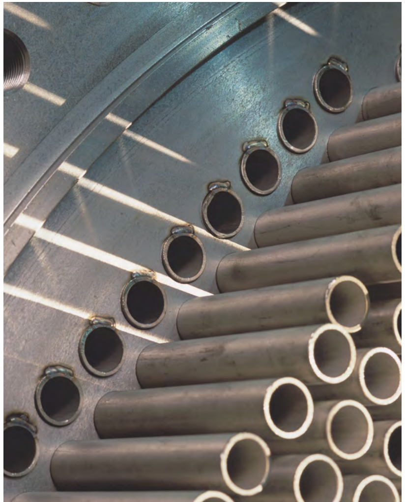
Heat exchanger tubesheet during fabrication. (Source: Sandvik)
