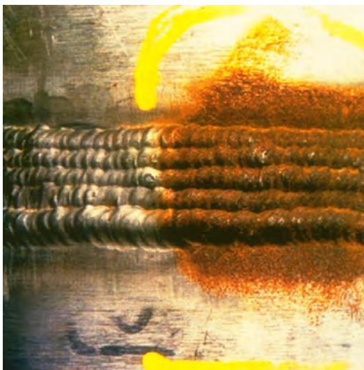
Carbon steel wire brushes used to clean stainless steel welds can produce discoloration and rust. (Source: Outokumpu Stainless)
