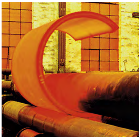
Hot roller bending of duplex stainless steel plate. © Outokumpu
