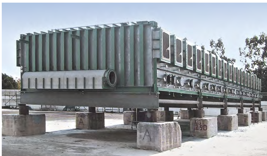
Multi stage flash seawater desalination unit constructed of S32101 and 2205 duplex stainless steels. © Outokumpu
