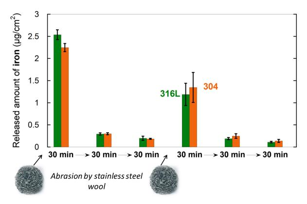
**Repeated exposure.** Released amounts of Fe upon repeated exposure of stainless steels 304 and 316L for 30 min at 100 °C in 5 g/L citric acid (pH 2.4). All samples were abraded with stainless steel wool, ultrasonically cleaned (in ethanol and acetone for 5 min), dried, and aged for 24 h (room temperature, in a desiccator) before the first and the fourth step of the exposure sequence.
