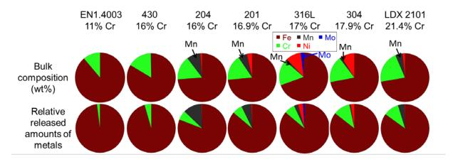
**Preferential release of Fe and/or Mn.** Nominal bulk composition (wt%) of all grades compared with the corresponding proportion of released metals after 240 h exposure (2 h at 70 °C, followed by 238 h at 40 °C) in 5 g/L citric acid (pH 2.4).
