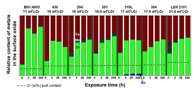
**Chromium enrichment in the surface oxide with time.** Oxidized metal content of the outermost surface oxide (2-5 nm) of as-received stainless steel surfaces (0), and after different exposure periods (up to 10 days) in 5 g/L citric acid (2 h at 70 °C followed by exposure at 40 °C for another 24 or 238 h).
